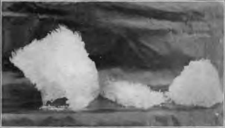
(c) Anchor Ice Removed From Champion Intake Screen.
